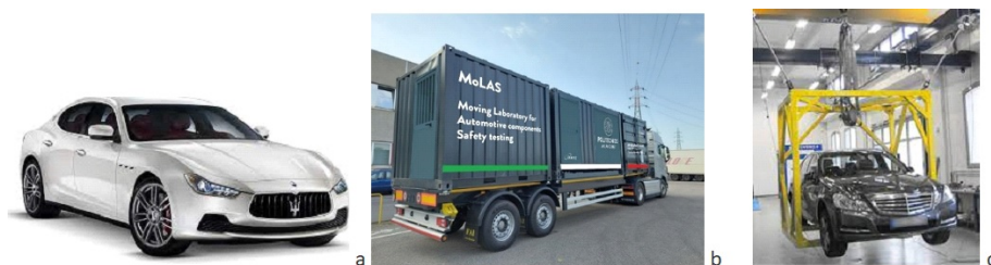
Fig.2. (a) Actual car taken into consideration (example). (b) Moving laboratory of the Politecnico di Milano to measure tyre characteristics, (c) InTenso system of the Politecnico di Milano to measure the mass properties of cars.
