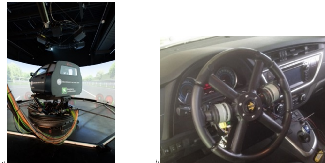
Fig.3. (a) DriSMi - Driving simulator of the Politecnico di Milano. (b) Instrumented steering wheel (ISW) able to measure the three forces and three moments at each hand, plus the grip (holding force) at each hand [44].
